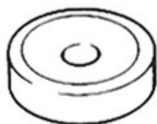
EP adapter (Fastened by tape to the top of the platter)
